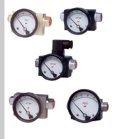
DIFFERENTIAL PRESSURE MONITORING : DK's Differential Pressure Instrument measures the difference in pressure at two Pressure zones in a system. Model GP-200 indicates the resultant differential Pressure [DP] directly on a single Gauge dial. This can also be equipped with 'Switch Actuation' mechanism, as an important additional feature.
